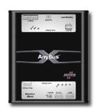
The Profinet IO interface is a complete solution for a Profinet IO slave Device. The module is based on the Siemens Profinet IO software technology.
